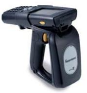
The IP4 Intellitag reader handle is a snap-on, high-impact plastic and magnesium trigger handle accessory that adds the capability to read and to write to RFID tags to all Intermec<sup>®</sup> 700 Series Color Mobile Computers.
