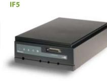
The IF5 Intellitag fixed reader is an intelligent RFID reader that can be factory configured to operate in RFID frequency bands: 869MHz or 915MHz. In addition to performing both read and write functions, the IF5 is also capable of running custom applications to filter information from tags, as well as monitor external sensors and control audible and visual indicators.
